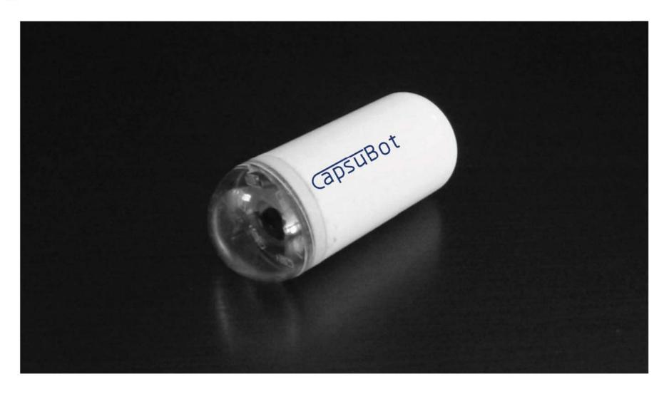
The high resolution capsule is consist of camera module, battery and wireless transfer chip which is a disposable product for small bowel diagnosis and screening.
